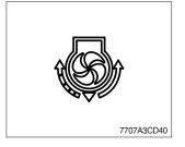
This lamp lights ON when the fan control switch is pressed.
