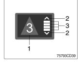
(1) The LCD can be used with the gear selector. It indicates speed and driving direction.
