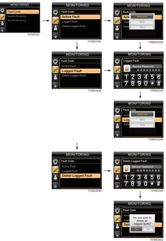
· Monitor the fault code of the Machine/ECU/TCU.
